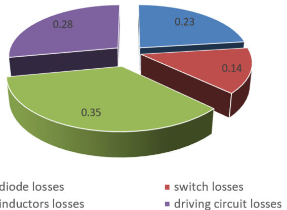
Fig. 31. Losses dissipation of the prototype.
