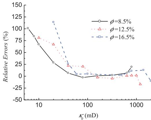
Figure 7 Relative errors in the permeability inversion by using the Stoneley wave of the acoustic logs, according to the data in Wu *et al.* (1995).
