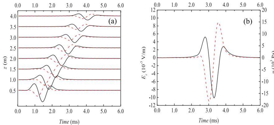
**Figure 2** Full waveforms of pressure  $p$  (dashed lines) and electric field  $E_z$  (solid lines) along the borehole axis of the seismoelectric logging in a sandstone formation with 1 kHz source centre frequency. (a)  $z = 0.5\text{--}4.0$  m (b)  $z = 3.0$  m.
