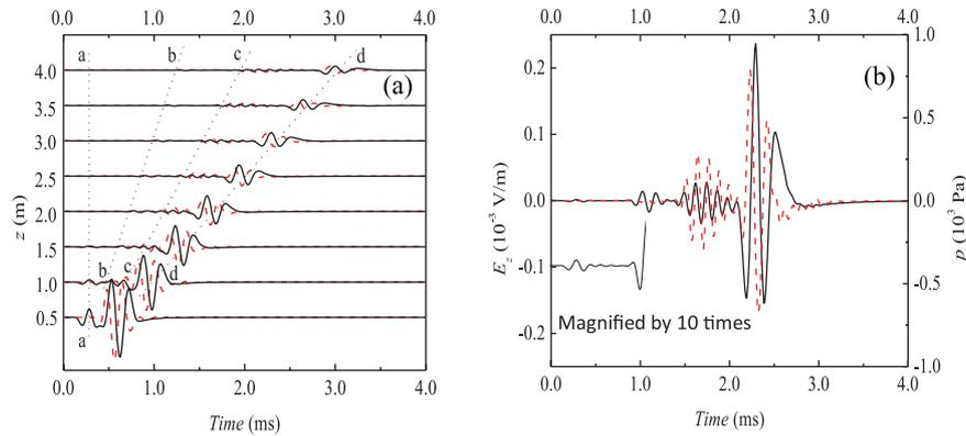
**Figure 1** Full waveforms of pressure  $p$  (dashed lines) and electric field  $E_z$  (solid lines) along the borehole axis of the seismoelectric logging in a sandstone formation with 6 kHz source centre frequency. (a)  $z = 0.5\text{--}4.0$  m, the dotted lines with a, b, c, and d denote four different wave groups in the full waveforms. (b)  $z = 3.0$  m.
