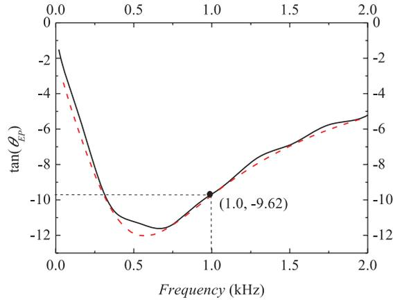
**Figure 5** Comparison of the tangent of the REP's phase obtained from the simulated full waveforms in Fig. 2(b) (solid line) with that obtained from the residue calculation method (dashed line).
