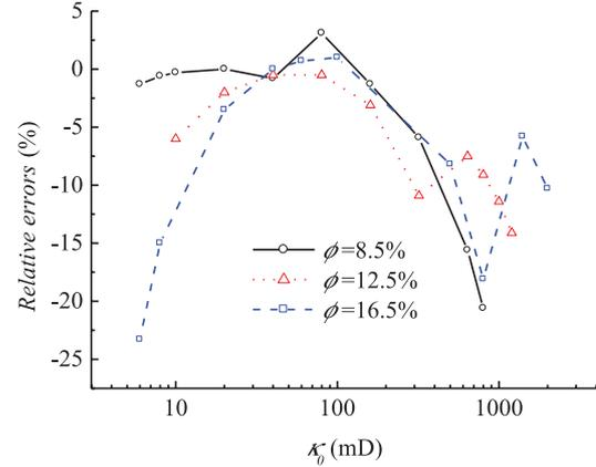
Figure 6 Relative errors in the permeability inversion by using the tangents of the REP's phase of the seismoelectric logs, according to the data in Table 3 and after correction.
