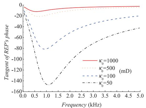
Figure 4 Frequency-dependent curves of the tangent of the REP's phase for different permeabilities of sandstones obtained from the residue calculations of the borehole pressure and electric field functions at the Stoneley wave pole.
