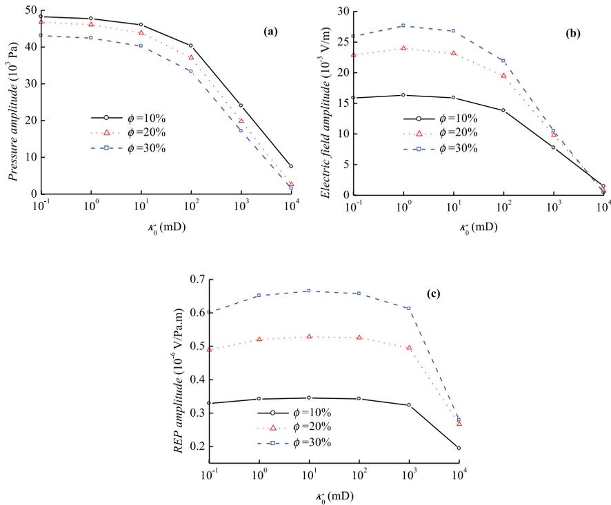
Figure 3 Amplitude variations of the pressure, the electric field and the REP with different porosities and permeabilities, according to the data in Table 2. (a) the pressure (b) the electric field (c) the REP.
