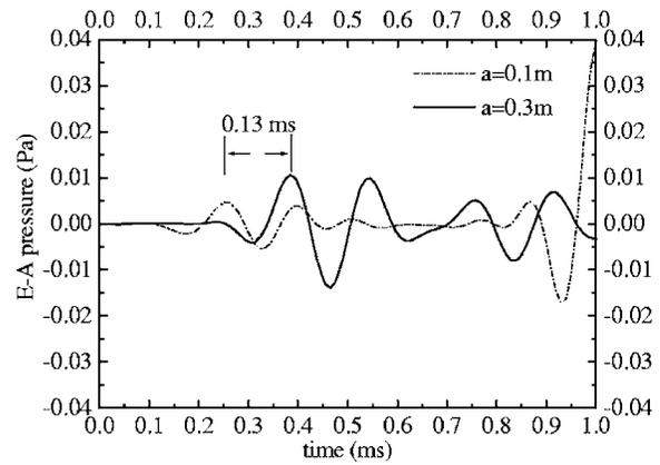
FIG. 3. Waveforms of E-A pressure  $p$  on the borehole axis at  $z=3$  m when the borehole radii are 0.1 and 0.3 m. Only waves in the first millisecond are shown. The earliest arrival delays about 0.13 ms when the borehole radius changes from 0.1 to 0.3 m.
