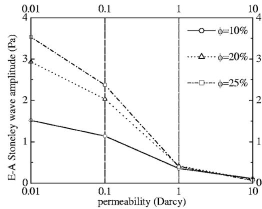
FIG. 6. Showing the amplitude variation of the E-A Stoneley wave with different porosities and permeabilities, according to the data in Table II.
