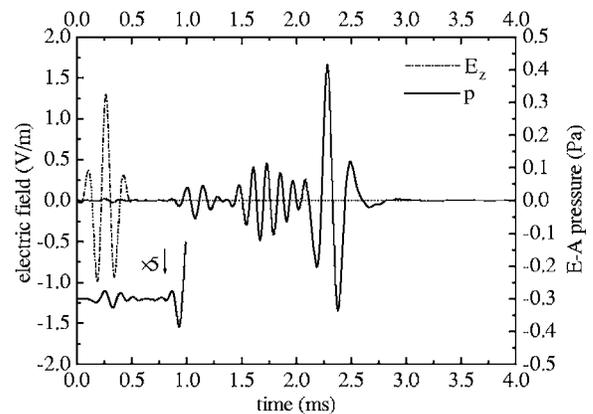
FIG. 4. Waveforms of E-A pressure  $p$  and electric field  $E_z$  on the borehole axis at  $z=3$  m. Also shown in the figure is the front part of the waveform of E-A pressure  $p$ , which is magnified by five times for the comparison with the waveform of electric field  $E_z$ .
