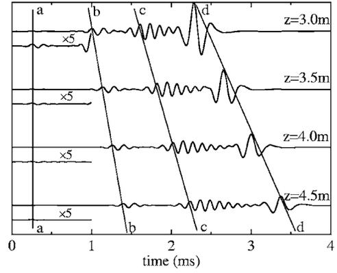
FIG. 1. Transient full waveforms of E-A pressure  $p$  on the borehole axis when the distance to the source  $z$  varies from 3 to 4.5 m. The waveforms are scaled to the wave magnitude at  $z=3$  m. The waveforms in the first millisecond are magnified by five times.
